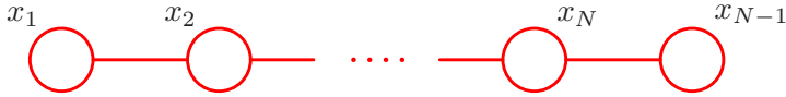
Fig. 12. A simple undirected graph comprising a chain of nodes, used to illustrate the solution of inference problems
