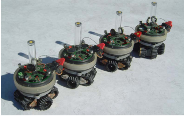
Fig. 2. A swarm-bot composed of four interconnected s-bots in chain formation
