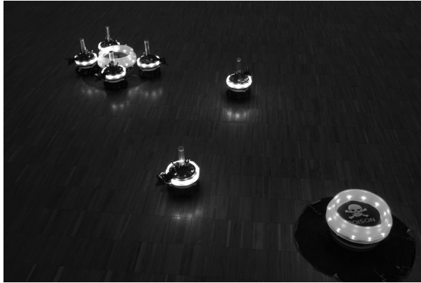
Fig. 7. A team of s-bots engaged in cooperative communication. A team of four s-bots feed on the food objects while they are lit up in blue color. Two s-bots in white color are attracted by the blue signal and move away from the poison object.
